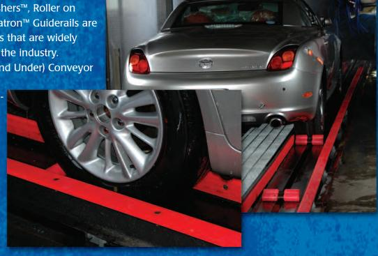
Hannatron high density polymer is attached to the conveyor guiderails to avoid scratching wheels and insure smooth travel. Hanna's Roller On Demand™ allows vehicles entering the carwash to stop, without interrupting the washing of vehicles in process. No wonder it is the industry's best selling conveyor.
